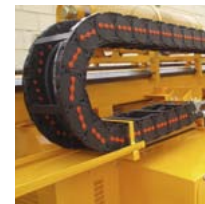
Nylon chain LC85 mounted on a drilling machine
